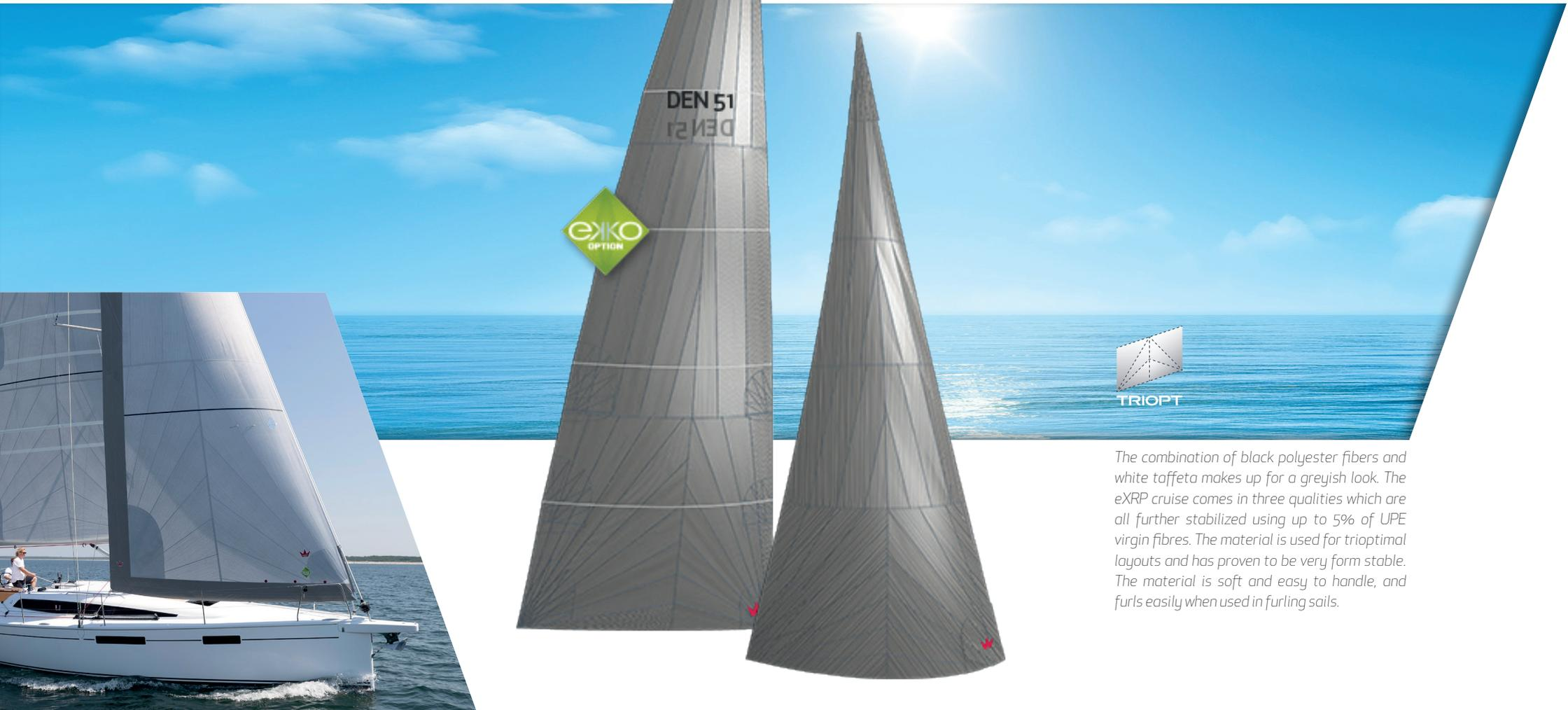
The combination of black polyester fibers and white taffeta makes up for a greyish look. The eXRP cruise comes in three qualities which are all further stabilized using up to 5% of UPE virgin fibres. The material is used for trioptimal layouts and has proven to be very form stable. The material is soft and easy to handle, and furls easily when used in furling sails.
